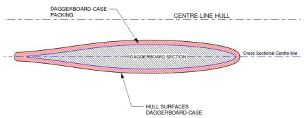
Advisory note: nowhere is re-finishing, fairing of the daggerboard casehull surface intersection permitted except to facilitate localised repair in this rule. Provided that the essential shape, characteristics and function of the original component are not affected, the N.S. may use templates to verify compliance with these limitations.
